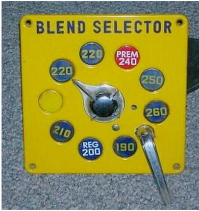
The good 'ol days... When we had REAL choices at the pump! This photo shows a blend selector from Sunoco's "Dial-A-Grade" pump, commonly found back in the '50's and 60's.
