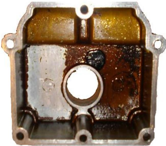
At left is an image of a carburetor float bowl from a 1967 Jaguar XKE. The tank of this car was filled with gasoline that was later determined to be a high RVP winter blend. It was parked in a climate-controlled garage for 20 months. The gasoline evaporated from the carburetor, leaving behind heavy, sticky gums. The gums were bad enough to prevent the carburetors from functioning, and the car would not start or run.
