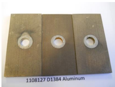
RO water with No-Rosion
